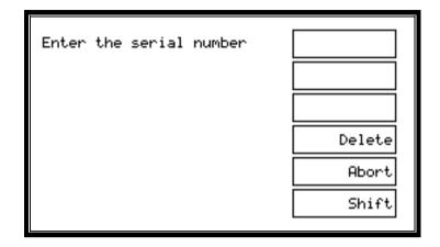
Use either the keypad or a barcode reader to enter the operator/batch/serial number, then press the ENTER key on the keypad or the 'Enter' softkey.
