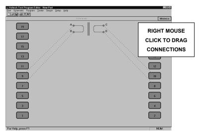
You have now created a schematic layout of a four-terminal transformer.
