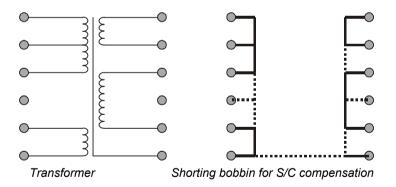
Put the short-circuit bobbin into the fixture and:
