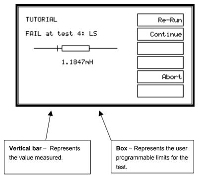
An example of this display for an inductance test is shown below.
