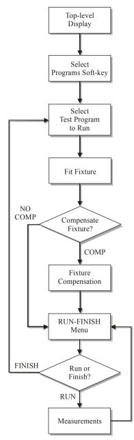
For simple test programs, (where none of the following options are enabled: batch number, operator number or serial number), the flow diagram shown on the left summarizes production mode operation. At the top-level display, press softkey 1 'Programs'.
