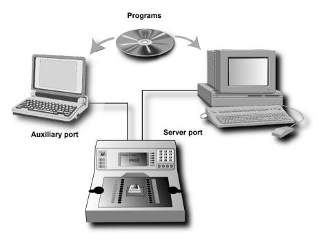
The standard installation uses separate PCs for the Editor and Server:
