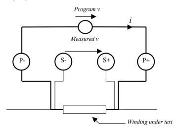
**Note:** The BNC connectors are also connected internally to nodes 20 (P+ and S+) and 18 (P- and S-) of the fixture bay.
