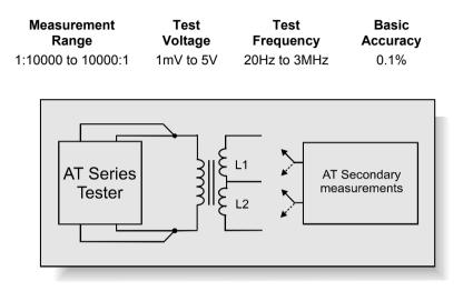
The inductance of a winding is determined by the number of turns and the construction and dimension of the core materials; it may also vary with test conditions such as voltage and frequency. See the LS and LP tests.
