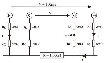
4-wire measurement circuit
