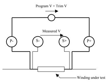
ATi basic measurement circuit
