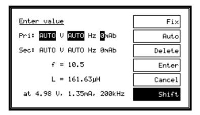
When the '**Shift**' key (softkey 6) is pressed, it is shown in reverse video. Press '5' with the '**Shift**' key in reverse to enter the multiplier k (x1,000). Press '6' with the '**Shift**' key in reverse to enter the multiplier M (x1,000,000).
