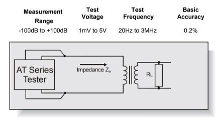
The return loss is a measure of the impedance mismatch between the transformer and a transmission line.
