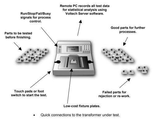
• Rapid change of fixture for different transformer types.
