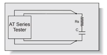
The parameter 'D' is most often used as a measurement of the losses in a capacitor. It is analogous to Q for a transformer winding.
