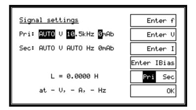
New settings are diplayed as above, once they have been stored. Since no measurements have been made with these new conditions, measured values cannot be displayed on bottom line.
