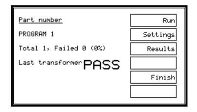
To change the batch number, press 'Settings', and the following display will be revealed. Choose the 'New Batch' softkey to enter a new batch number at this time, or to change the operator name, press the 'Operator' softkey.
