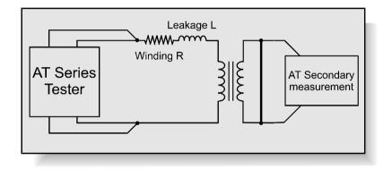
Due to imperfections in the coupling between windings, a short-circuited transformer acts as if there is inductive impedance in series with the winding. This impedance is known as the leakage inductance. Low leakage inductance implies good coupling; high leakage inductance, poor coupling.
