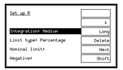
Use the arrow key to scroll through and set up the test parameters. For example, to set up limits, scroll to the 'Limit type' line and press softkey 3 three times to enter both minimum and maximum limit values.
