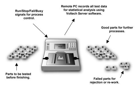
Again, the tester may be connected to a Server PC or used stand-alone, as described above.
