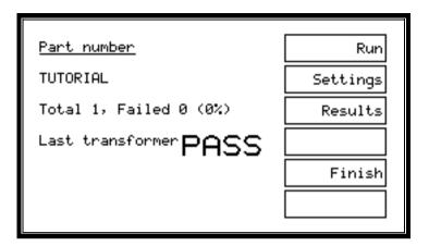
Press the RUN softkey several times to repeat the program execution. On each run of the program, the test results should be passed back to the Server, where they may be viewed in the 'On-line Monitor' window
