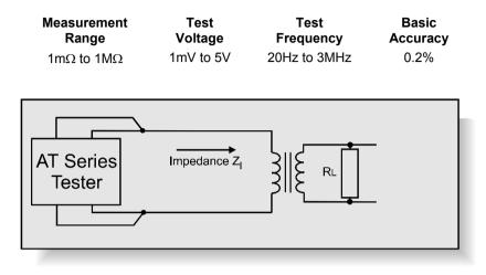
The impedance of a transformer is usually complex, that is it consists of real (resistive) and inductive or capacitive (imaginary) parts. The total impedance at a specified frequency is the vector sum of these parts.
