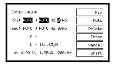
Press '**Fix**' to enter the value currently being measured by the ATi. (This does not apply to 'IBias', the DC bias current.)
