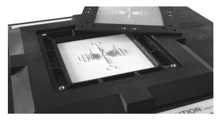
Example probe box drilled for multiple RM bobbin types
