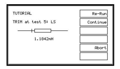
The main difference between this and the 'Stop on fail' display is that the reading on the fourth line will be continuously updated, allowing adjustments to be made to bring the test result within limits.
