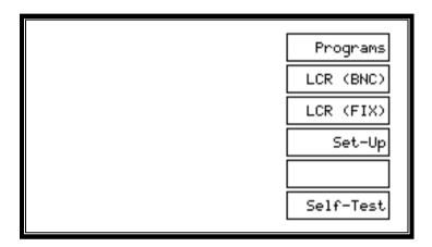
To access set-up mode from the top-level menu (see above), press the 'Set-Up' softkey to change to the following display:
