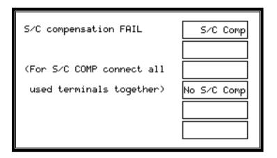
Should either S/C or O/C compensation display a FAIL, as shown above, check:
