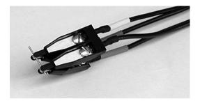
To perform open-circuit compensation for stray capacitance, remove all parts under test but leave the BNC leads or test fixture in place and press softkey 2 'Open' and select '**One**' or '**All**'.For optimum accuracy, place any leads or other connectors that can move in a position as close as possible to that which will be used when making measurements.
