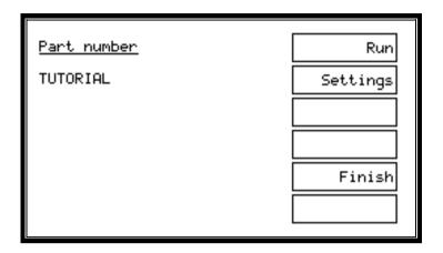
Running the program will take you to the PASS/FAIL display, where pressing 'Finish' will return you to the program selection screen, where you may choose to re-run the test program, run a different test program, change the set-up of am existing test program, delete a program or create another, new program from the front panel.
