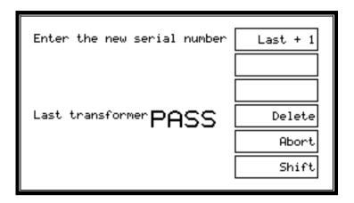
If the next serial number to be used simply follows on in sequence after the previous one, then press the 'Last + 1' softkey (or the touch pads). This will enter the next serial number automatically and return the display to the RUN-FINISH selection.
