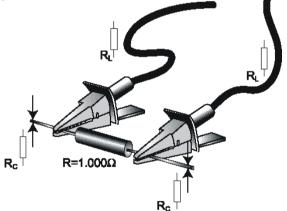
$R_L$ , the resistance of the leads, is fixed and can be compensated for. Let's assume it is  $2m\Omega$  for good quality leads.
