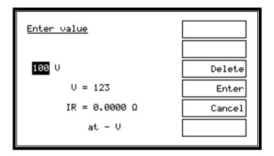
Enter the required test voltage using the 12-key numeric keypad.
