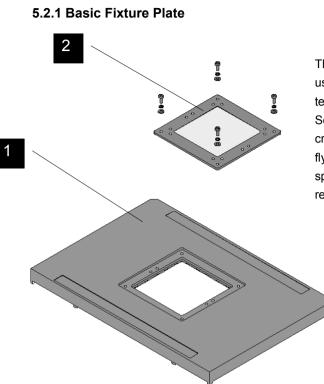
The fixture plate may be used to mount existing test fixtures onto an AT Series Tester or to create test fixtures for flying lead parts where spring probes are not required.
