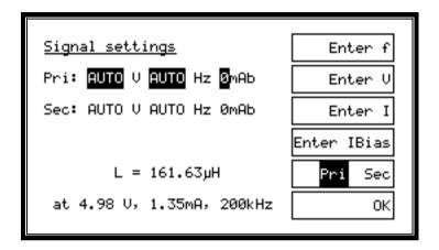
Note that in LCR (BNC) mode there is only one set of conditions to choose and that the 'Pri Sec' softkey is thus not shown. On the bottom line of this display, the last measurement and its measurement conditions are displayed, if they are available.
