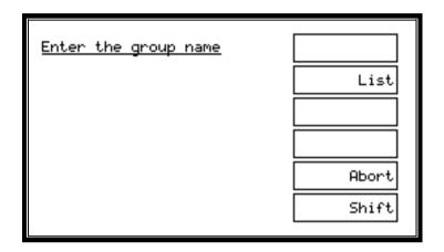
As with other names, the group name can now be typed in from the keypad, entered using a bar-code reader connected to the bar-code port of the ATi, or selected from a list using the 'List' option. (Again, the cursor softkeys and the 'Delete' softkey may be used to correct errors.)
