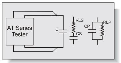
The CS and CP tests can be used to measure the capacitance of a wide range of components up to 1 milli-farad.
