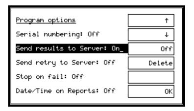
Once you have completed the program options set-up, press 'OK' to return to the program test selection screen and 'OK' again to confirm your set-up. Note that, if a password has been set, the AT requests the password to be entered before the program can be saved.
