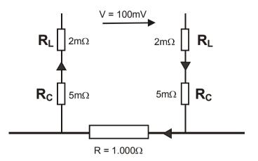
2-wire measurement circuit
